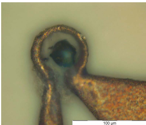
FIG. 8. (Color online) Photograph of the 50 \mu m R-shaped PMR with a DPPH grain in the center of the loop.
