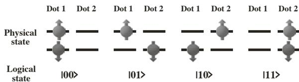
Figure 12.30: Possible encoding of two qubits by a single electron–hole pair in two quantum dots. State  $|0\rangle$  is identified with the particle being in dot 1, state  $|1\rangle$  with the particle in dot 2.
