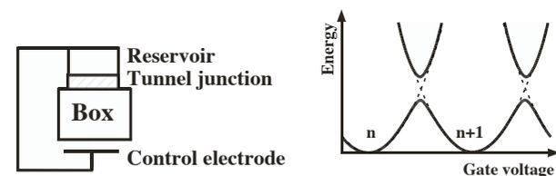
Figure 12.23: Components of a superconducting qubit (left) and its lowest energy levels as a function of the gate voltage (right).
