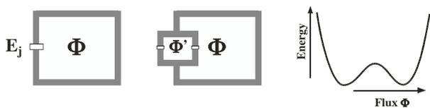
Figure 12.24: A simple flux qubit (left) consists of a loop that includes a Josephson junction. The second version allows control of the Josephson energy by the flux  $\Phi'$ . The total energy forms a double well potential as a function of the flux.
