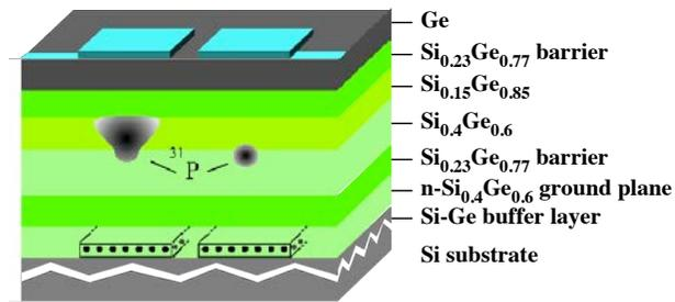
Figure 12.7: A proposal for a  $^{31}\text{P}$  qubit on the basis of a SiGe heterostructure.
