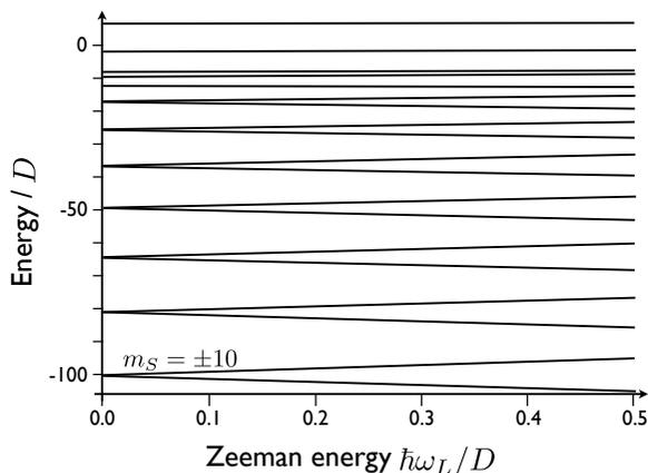
Figure 12.17: Energy levels of an  $S = 10$  system, corresponding to the Hamiltonian (12.1), with  $E/D = 0.05$ .
