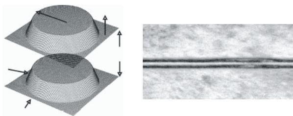
Figure 12.28: Two coupled quantum dots as qubits; left: schematic representation; right: transmission electron micrograph; height of dots is 1–2 nm, dot separation 4 nm, dot radius 8–12 nm [318, 319].
