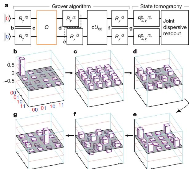
Figure 12.26: Grover algorithm implemented with 2 superconducting qubits.[313]
