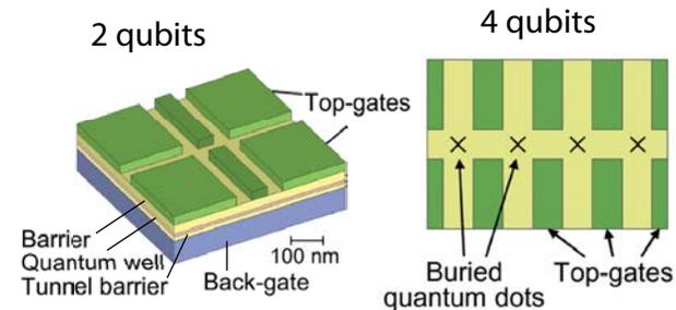
Figure 12.8: Electrostatically confined electron qubits in a Si/SiGe quantum well.
