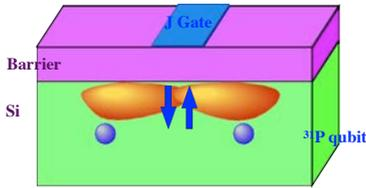
Figure 12.5: Principle of operation of J-gates.
