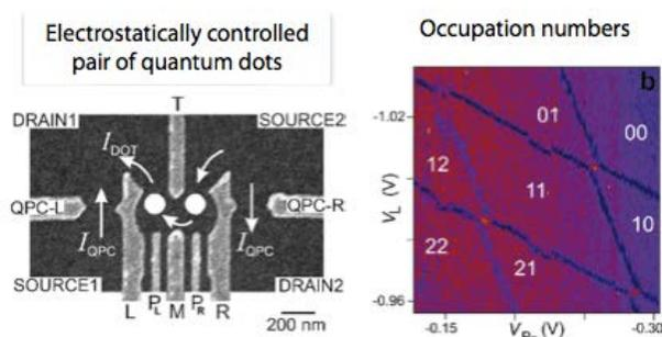
Figure 12.29: Electrostatically defined quantum dot pair. [320]
