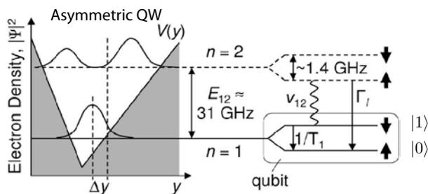
Figure 12.31: Readout scheme for a spin-qubit in an asymmetric quantum well.[345]
