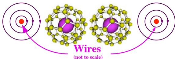
Figure 12.10: Scheme for resonant addressing of  $N@C_{60}$  molecular spins: the wires carry copropagating currents, which shift generate a magnetic field gradient superimposed over a static external magnetic field.
