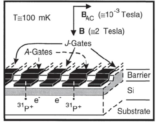
Figure 12.2: Proposed scheme for a quantum computer that uses  $^{31}\text{P}$  atoms in a  $^{28}\text{Si}$  matrix [239].
