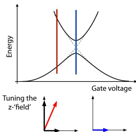
Figure 12.25: Gate operation for a charge qubit.
