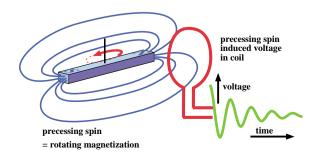
Detection in magnetic resonance is best described in a classical picture: the transverse components of the spin generate a macroscopic magnetisation that precesses around the static magnetic field. The magnetic flux through a coil oriented perpendicular to the field changes therefore sinusoidally. According to Faraday's law, such a temporal variation in the magnetic flux induces a voltage in the coil, which is recorded as the signal.
