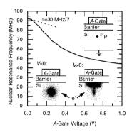
The hyperfine coupling between electrons and nuclei would depend on the position of the electrons. These so-called A-gates could therefore be used for addressing the individual qubits. Similarly J-gates would move electron density between the donor sites, thus inducing an indirect coupling between qubits and allowing the addressing of pairs of qubits.
