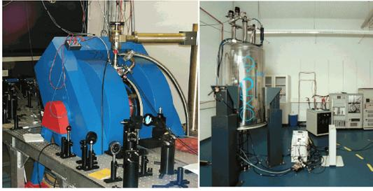
$B_0 = 1.4 \text{ T}$     $\omega_0 = 60 \text{ MHz}$     $B_0 = 14 \text{ T}$     $\omega_0 = 600 \text{ MHz}$
