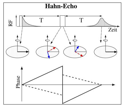
$$\rho(T) = \sum_{i} (\cos(\Delta \omega_{o}^{(i)} T) S_{x}^{(i)} - \sin(\Delta \omega_{o}^{(i)} T) S_{y}^{(i)}) e^{-\Gamma_{2} T}.$$
