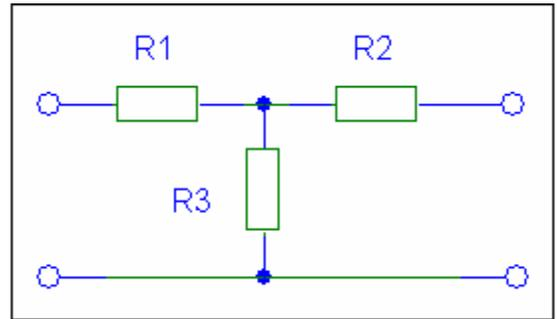
$R1 = 1.5 \text{ k}\Omega$ ,  $R2 = 1.5 \text{ k}\Omega$ ,  $R3 = 3.3 \text{ k}\Omega$
